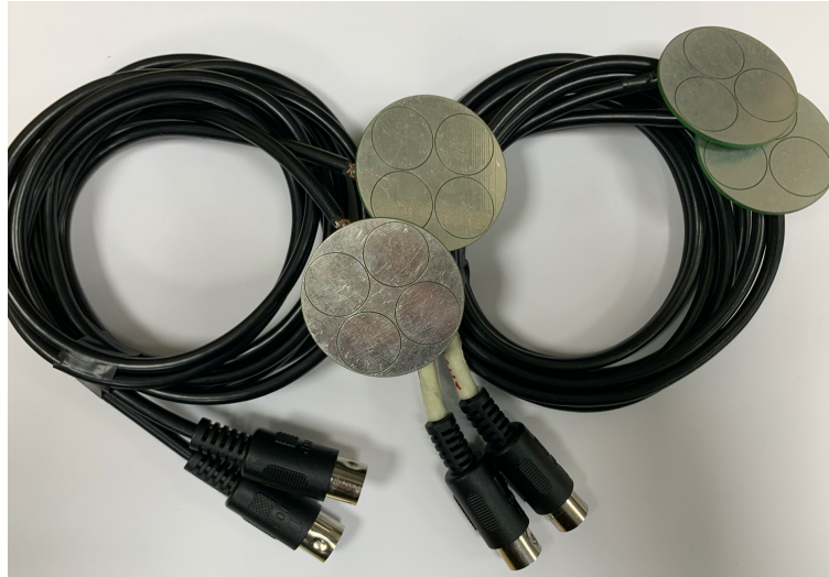
Figure 4.32 - Multi-sensor electrodes fabricated PCBs
