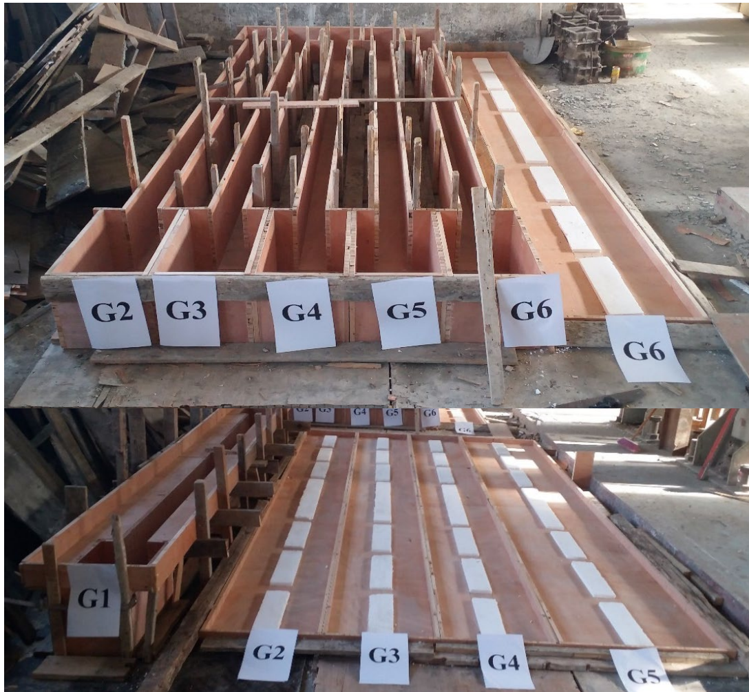
Figure 7: Preparation of formwork for tested specimens
