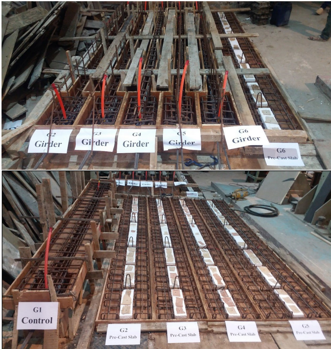
Figure 9: Finishing preparation of reinforcement for all specimens
