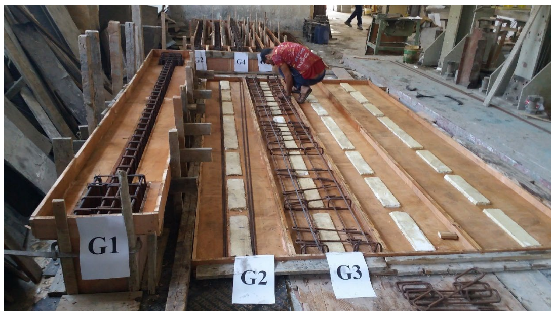
Figure 8: Preparation of reinforcement for tested specimens
