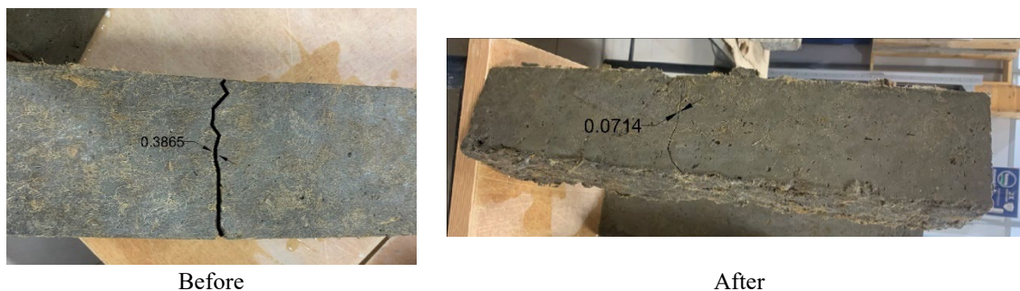
Fig. 10. Crack closure of prism specimens at initiating cracks and after applying the healing process at 28 days of age for mix BC + PVAC1
