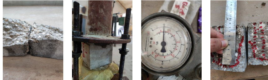
Fig. 13. A typical cube specimen under sorptivity testing [79, 80]
