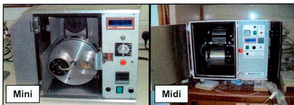
Figure 2.2: Countercurrent chromatography apparatus with maximum operating volumes of 100 \mu L (Mini) and 50 mL (Midi). Machines manufactured by Brunel Institute for Bioengineering, Brunel University.
