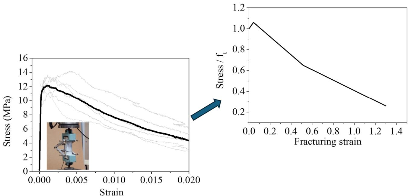
**Figure 4.** The experimental results of the direct tensile tests and the respective constitutive model [35].
