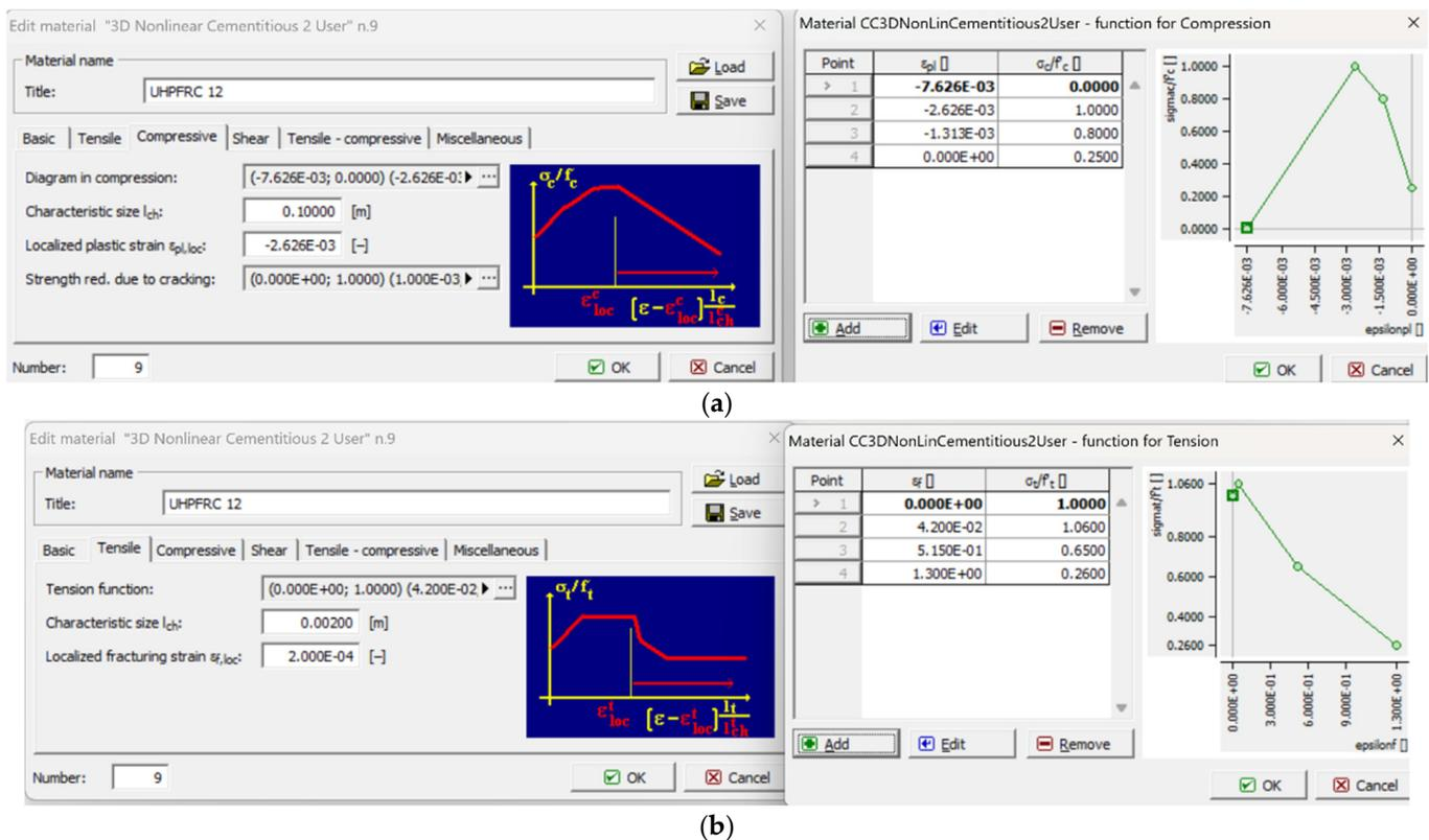
**Figure 5.** UHPFRC material model properties for (a) compression and (b) tension used for the numerical analyses of this study.
