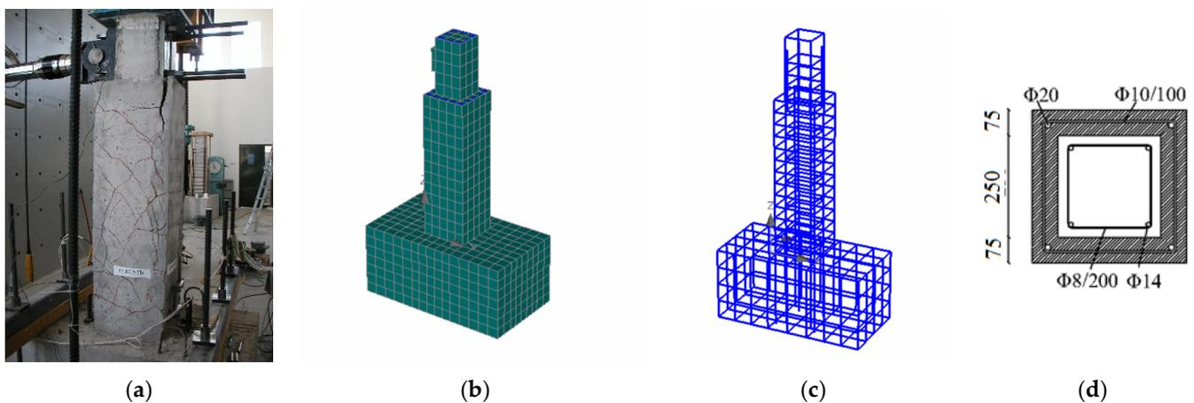
**Figure 1.** (a) RC-jacketed column tested in lab [14], (b,c) numerical models for concrete and for reinforcement, and (d) cross-section of strengthened column (dimensions in mm).
