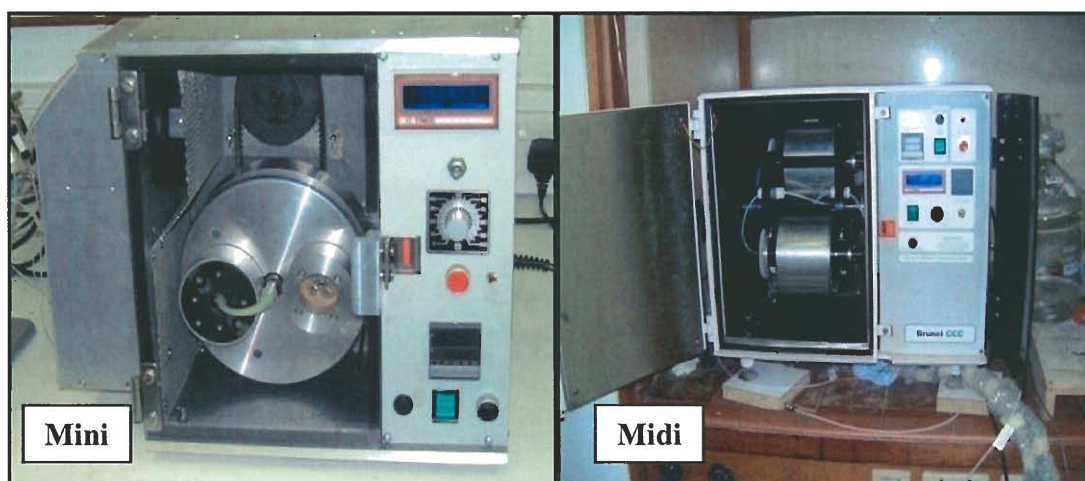
Figure 2.2: Countercurrent chromatography apparatus with maximum operating volumes of 100 \mu L (Mini) and 50 mL (Midi). Machines manufactured by Brunel Institute for Bioengineering, Brunel University.
