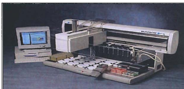
Figure 2.1: Liquid handling robot used for selecting solvent system ratios based on heptane, ethyl acetate, methanol, butanol and water
