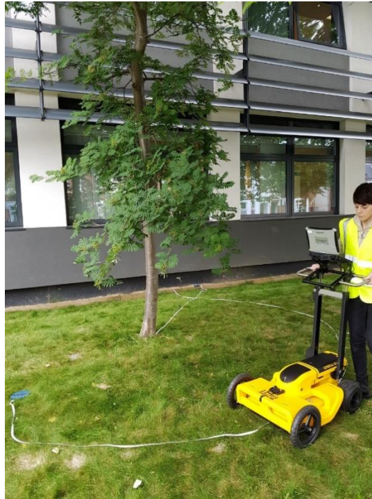
Figure 95: Opera Duo GPR system by IDS Georadar (Part of Hexagon) deployed in the survey of the ash tree.
