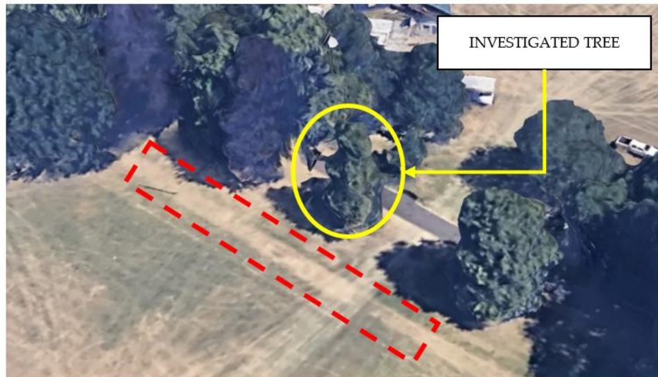
Figure 80: Aerial view of the investigated area. The red dashed area highlights a difference in the ground appearance matching the identified location of the discontinuity feature.
