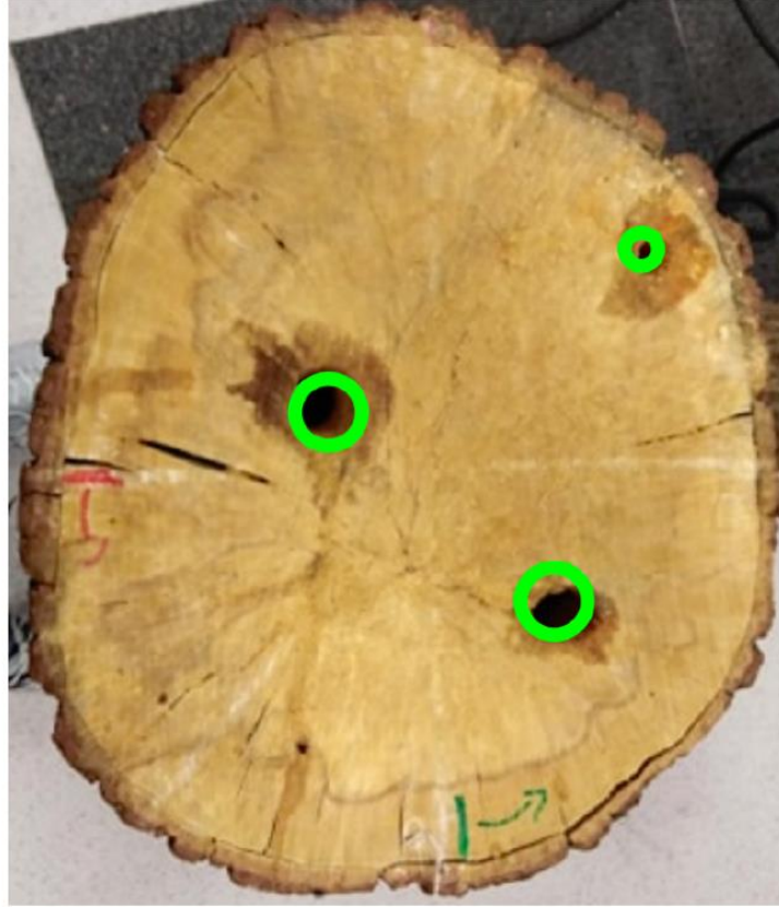
Figure 29: The estimated coordinates and radii of the decays using the proposed detection scheme are illustrated with green circles. The holes in the tree were filled with saturated sawdust during the measurements (see Figure 27). The holes are plotted empty in the current figure for comparison purposes.
